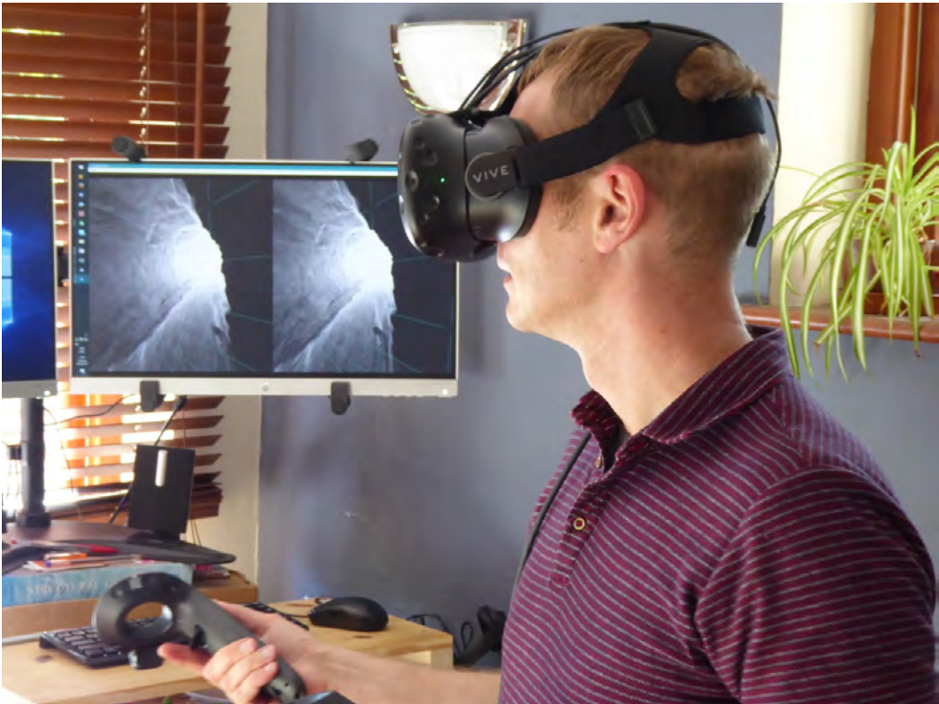
Figure 1: Using a Virtual Reality headset. Stereoscopic images of the multi-millions of points on the screen in the background are combined into a single 3D virtual world in the headset's eyepieces.
