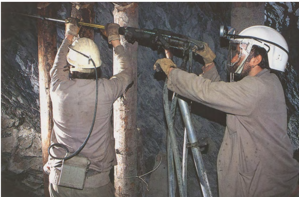
Introduction of the new Rascal airstream system powered protective helmets against mercury vapours and silica dust in 1983. (Photo: B. Kladnik, Archive: CUDHg Idrija)
